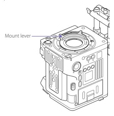
Place the PL lens adaptor back in its original position, insert the six hex screws (2.5 mm), and tighten the screws to a tightening torque of  $0.8 \pm 0.12$  N·m using a hex wrench (2.5 mm).
